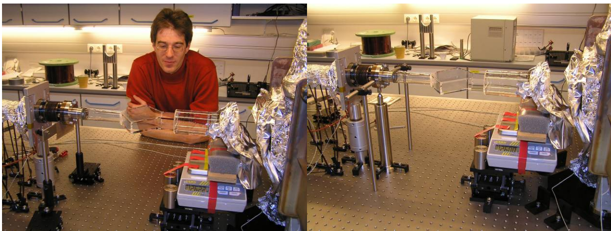
Fig. 4: replacing the entrance port clamp by the spring loaded rod.
