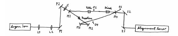
Figure 1: Setup of the Argon Ion pumped Ti:Sapphire ring cavity laser.
